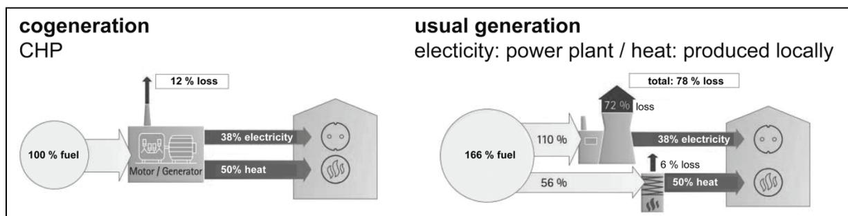
Figure 2: Comparison of CHP and usual generation of electricity and heat [7]
