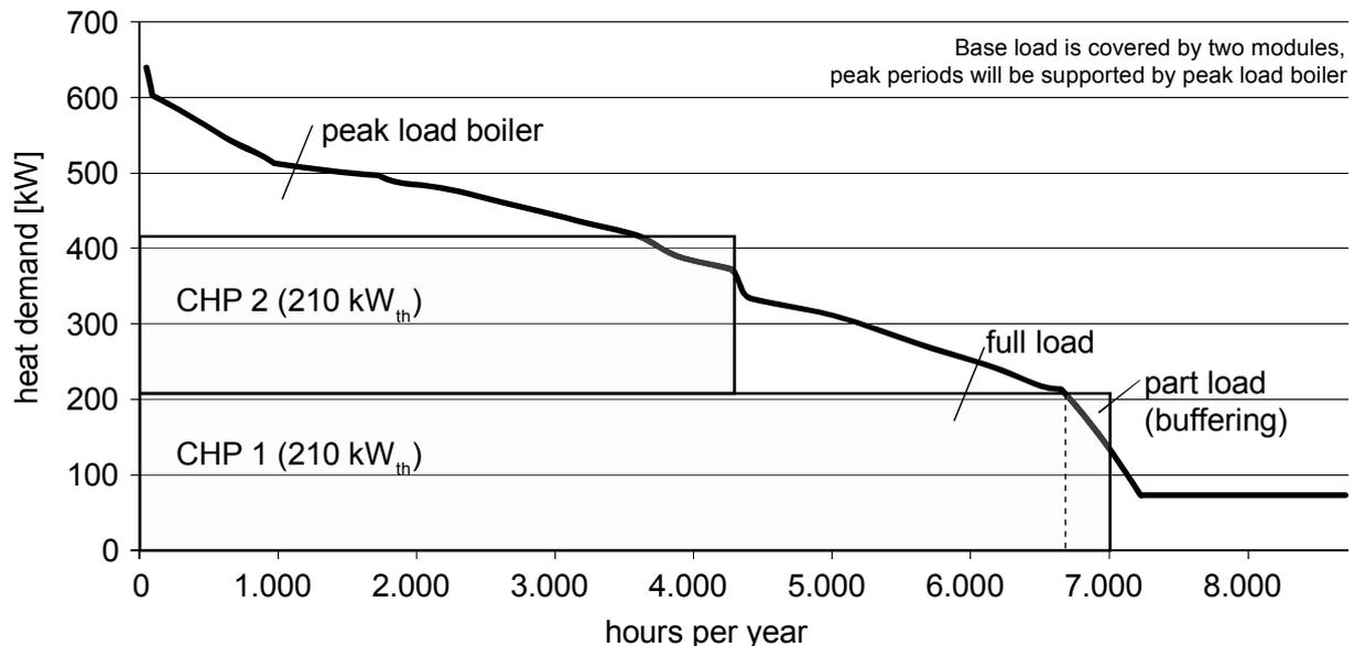
Figure 3: Annual load duration curve of power to be provided (example, heat led) [7]
